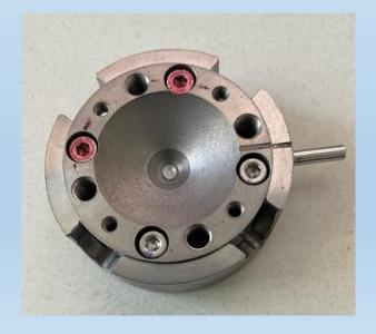
Unique cell with a physical angle of 120 degrees on both sides, particularly suited for single crystal diffraction.
